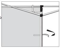
**NOTE:** straps fit best when velcro<sup>TM</sup> strips are aligned flush to one another.
